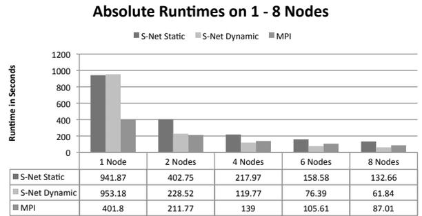
**Figure 14.** Runtimes of a Distributed S-NET-parallelised ray tracer with C-implemented boxes compared with a hand-coded MPI-implementation using identical sequential building blocks
