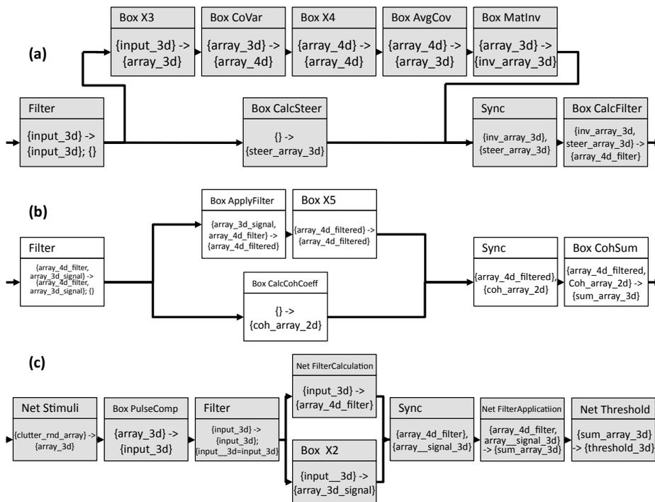
Figure 6. (a) shows network 'FilterCalculation'; (b) shows network 'Thresholding'; (c) shows the final MTI application.
