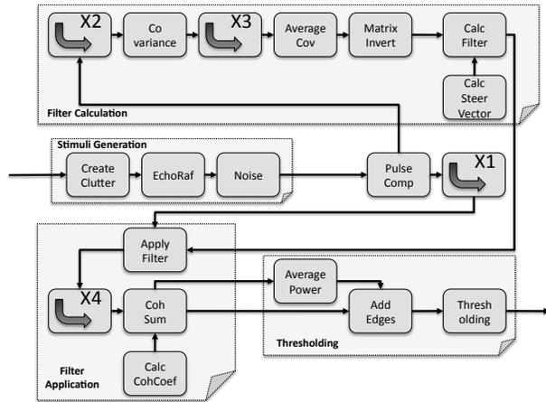
**Figure 4.** The data processing graph of the MTI application is subdivided into several modules. Modules are indicated by boxes with folded bottom right corners. Small boxes with text denote processing functions, boxes containing an arrow and a capital X with a number denote structure transformers. These boxes are used to re-arrange data in a matrix without effecting the actual values.
